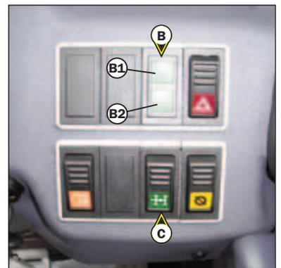
**⚠ Before driving on roads, it is necessary to check the alignment of the rear wheels and to drive in front wheel steer. The control of the alignment of the rear wheels must be regularly done with the help of the green lamps, while driving the lift truck. In case of anomalies, consult your dealer.**
