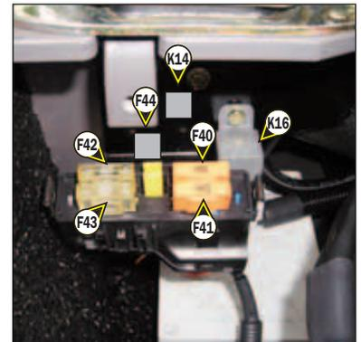
Remove casing 1 and cover 2 for access to fuses F40 to F44 and to relay K16.
